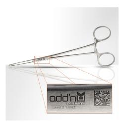
Annealing marking on stainless steel medical scissors, reprocessed 500 times. The UDI marking is still clearly readable, as the appropriate laser marking parameters in combination with a passivation provide long term protection against corrosion or fading and make the marking long-term resistant.
